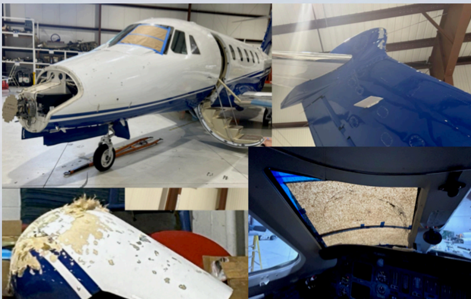
NTSB docket photos documented considerable skin, windscreen, and leading edge damage.
